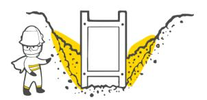
In loose soil shoring may also be necessary at depths less than 2 m.
