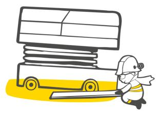
Check that the lift and any supporting legs are standing on a firm, level surface before use.
